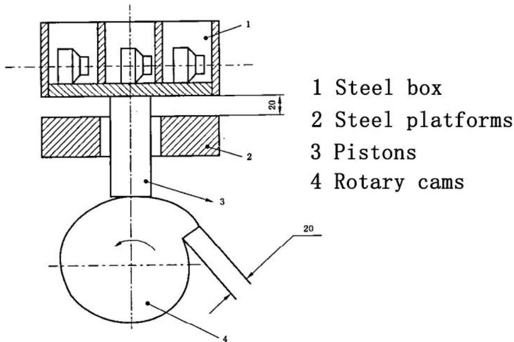
Figure 1: Schematic of the vibration test device
