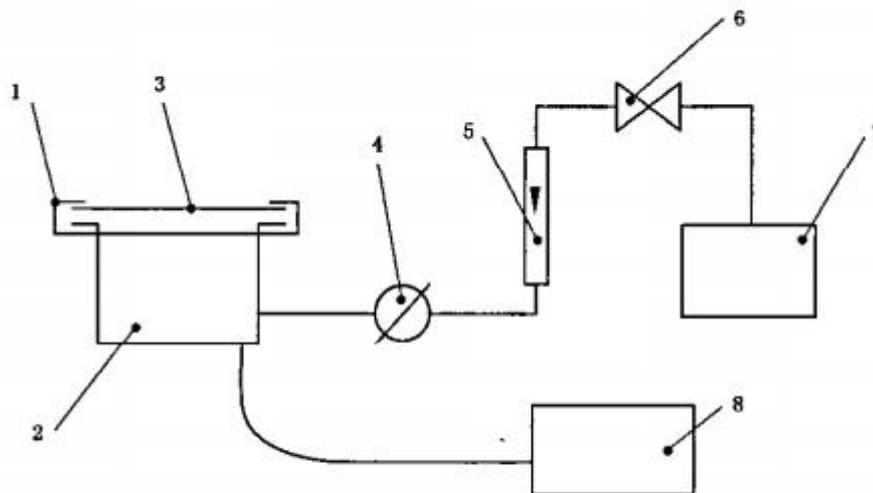
1 Breath valve fixture 2 Fixed cavity
